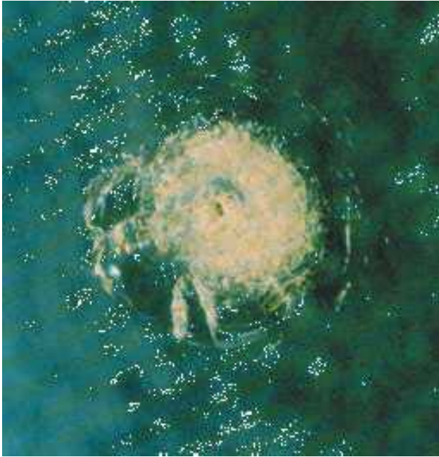
The space shuttle window after being hit by a flake of paint
